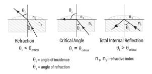
The critical angle can be used to easily calculate the refractive index according to the equation:
